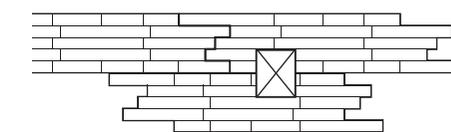
Light switches and power sockets can be integrated by cutting a hole within the panel. Always measure carefully before cutting the hole.
