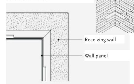
In case of an internal corner a seamless unbroken row of panels is achieved by joining corresponding panels using a mitered edge. Connect the return wall using the leftover piece from the joining panel.
