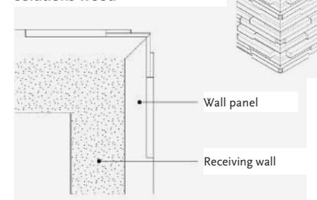
A seamless corner/unbroken row of panels is achieved by joining corresponding panels using a mitered edge. Connect the return wall using the leftover piece from the joining panel.
