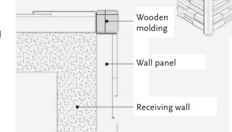
Using a square wooden molding will delineate joining walls and put a strong emphasis on the corner itself. We recommend that you use a well matched wood type for this solution.
