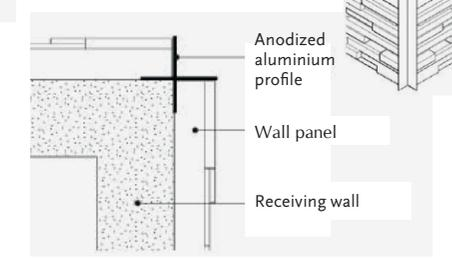
For this open corner solution we recommend using an anodised or powder coated aluminium profile of 2" x 2".
