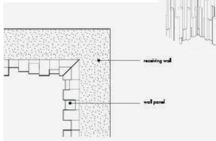
If a vertically placed corner solution is preferred we recommend one row of the wall panel overlap so the side of one for the panels is visible.
