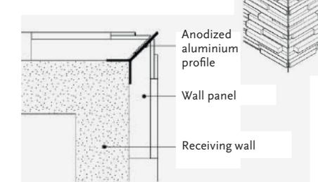
If a narrower, corner-defining solution is preferred we recommend using an anodised or powder coated aluminium profile of 3/16" thickness, positioned within the miter joint.
