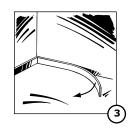
the walls. Flat skirting boards can be glued to the floor panels. Because wood naturally expands when it gets wet and shrinks when it is dry, you should always leave a (an expansion) gap between the wall and your Solidfloor, which gap is equal to the thickness of your floor panel. For that reason, floors with a thickness of
