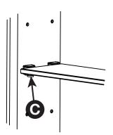
be positioned accordingly by sliding the supports up or down (NOTE: Take care to use both hands when sliding shelves and ensure that support brackets at both ends slide simultaneously). **9.** If the doors are out of alignment first remove the soft-close buffer (from the relevant hinges) which clips into the main hinge plate. The soft-close hinges offer adjustment in 3 directions via adjustment screws **D** and **E** (see diagram).
