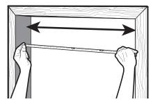
the opening is less than 80" high, the door may be shortened by sawing the excess from the bottom of the door panels.
