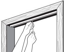
tighten. (Tape may be used to hold the track in place while you mark and drill.)
