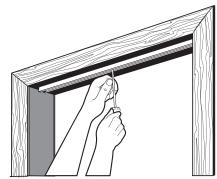
of the track. Do not fully tighten. (Tape may be used to hold the track in place while you mark and drill.)
