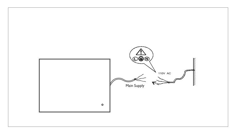
The next step is to make the electrical connection from the mirror to the mains supply. Use the connection wire found at the rear of the mirror to make the necessary connections. A second person will need to hold the mirror in place while electrical connections are made.
