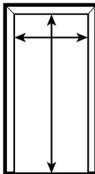
If the opening is less than 80" high: Stack the door panels together, secure with masking tape and cut with a hacksaw or fine tooth saw. Remove the masking tape. Cut the Top track 1/8" shorter than the width of the opening.
