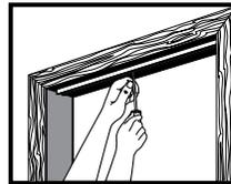
After making a screw pilot hole (with a nail or 3/32" drill), drive a 3/4" track screw through the screw hole nearest the center of the track. Do not tighten. (Tape may be used to hold the track in place while you mark and drill.)
