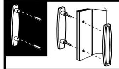
If necessary, you may back one handle with a solid object and tap the other handle alternately over each pin area until the handles are seated. Do not strike the middle of either handle.
