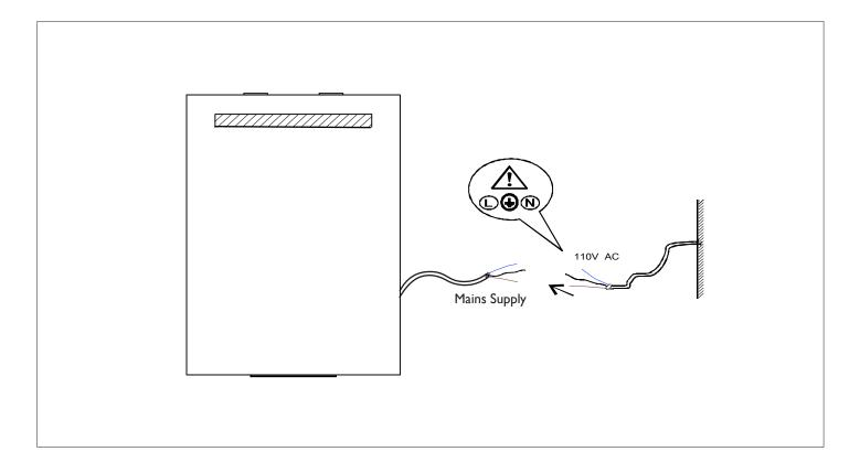
The next step is to make the electrical connection from the mirror to the mains supply. Use the connection wire found at the rear of the mirror to make the necessary connections. A second person will need to hold the mirror in place whilst electrical connections are made.
