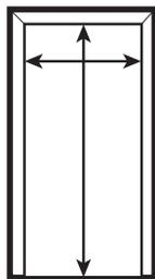
If the opening is less than 80" high: Stack the door panels together, secure with masking tape and cut with a hacksaw or fine tooth saw. Cut the overhead track 1/8" shorter than the width of the opening. Remove the masking tape.
