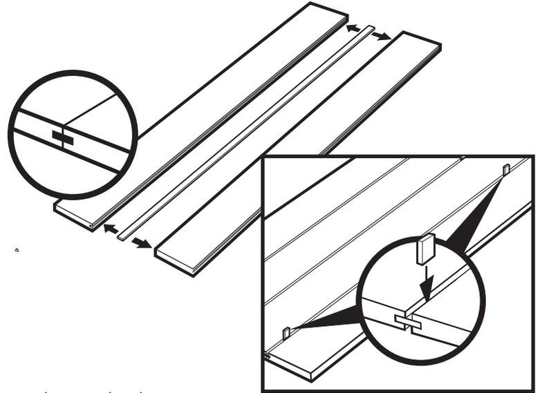
Make sure the door is square by measuring diagonally from both directions. These measurements must be equal. Using the mallet or hammer, adjust the boards until equal. Do not hit the splines. Remove the spacers.
