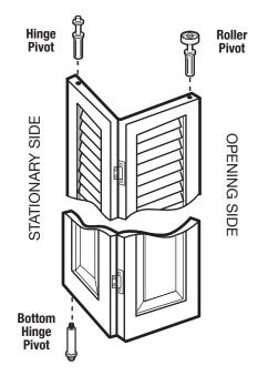
**Insert the bottom pivot.** This should be installed into the pre-drilled hole at the bottom edge of the door that will remain near the jamb side of the opening.
