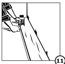
3. If the wall is not fully straight, you should transfer the unevenness to the floor panels. This may be done using a spacer with a lead pencil (see 12). After the floor panels have been marked out, saw the same as required so that the recesses, etc., fit together. Keep in mind the expansion joint. Use a fine-toothed saw for this purpose. If a hand saw is used, make sure the décor side is facing upwards; if a jigsaw is used, keep the décor side facing downwards (see 13).
